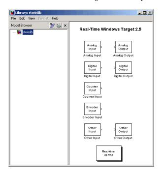
2 Click and drag the Analog Input block to your Simulink model. Remove the Signal Generator block and connect the Analog Input block to the Transfer Function block.
